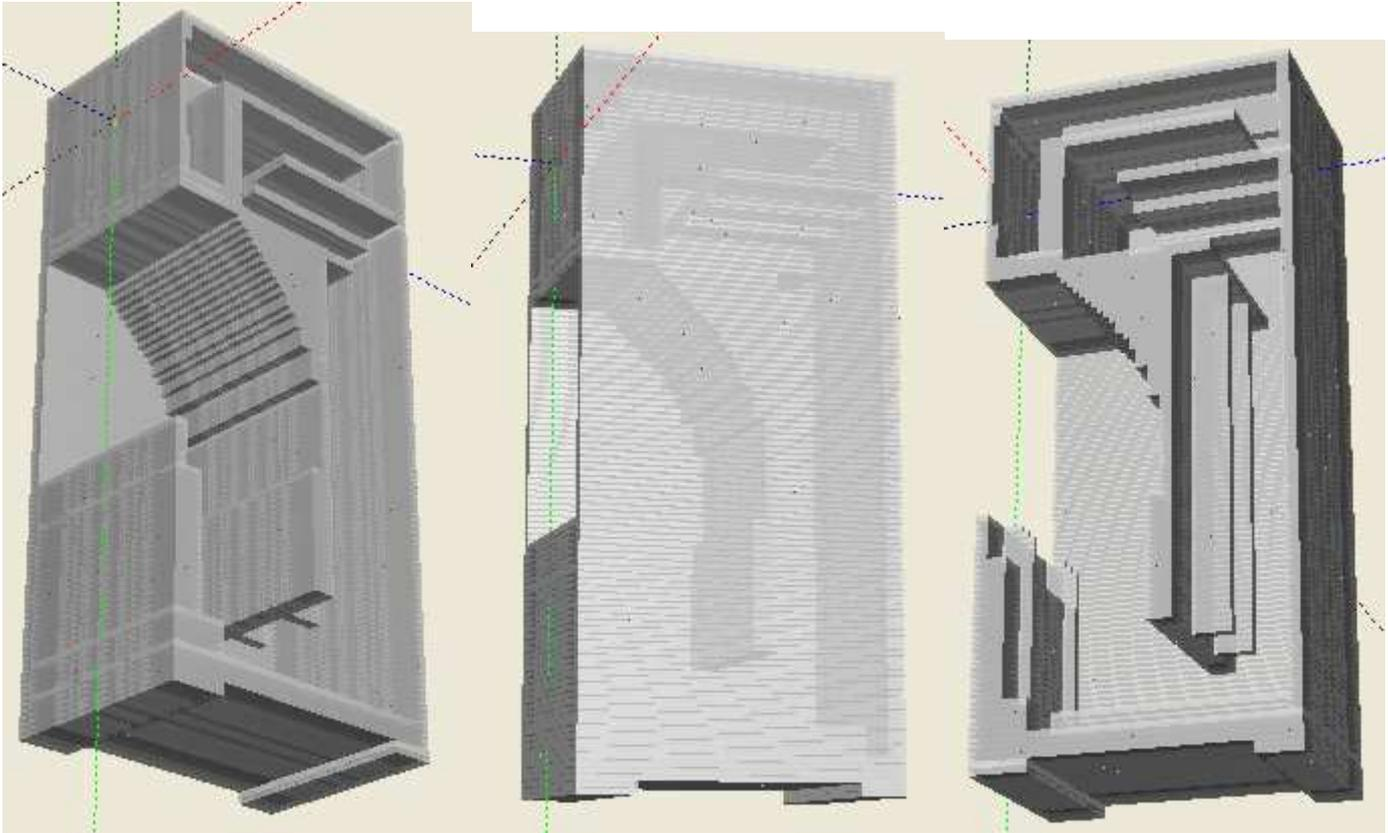
Fig.3 3D View of horn imported to Response 3D
